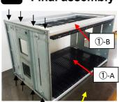
Please lay the 2 assemblies sideways as picture below. %Please make sure to put it sideways so as not to pinch your hand with 1)-B Guide rail unit B (movable side).
